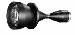
**Optical Specifications** Magnification (x) 0.393 Object Field of View (0mm) 150 Working Distance (mm) 300±5 Max Sensor Size (Фmm) 59 Best Aperture (F/#) 19.8 <0.1 Telecentricity typical (max) (deg) Distortion typical (max) (%) <0.1 MTF30 (lp/mm) >45 Depth of Field (mm) ±5.1@F20
